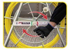
**3.** If, during the feed-in process a blockage or restriction is met then gently re-try by drawing the rod back a metre and reinserting. Using a stabbing action or forcing the rod could damage existing equipment in the channel. If this fails, try feeding the rod from the other end of the run. Once the rod is at a desired position, re-tighten the parking brake with clockwise rotation so the reel will not rotate in the frame.
